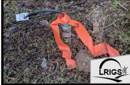
Soil heated to >150 °C to reduce contaminants, aka a soil oven
