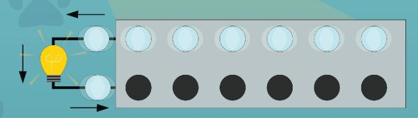
Different materials in solar cells require different amounts of energy to release electrons. Some only require a little energy, so most of the light rays will work. Others require lots of energy, so only light rays with more energy work. The best solar cells are designed to absorb the most abundant types of photons produced by the sun, including photons that we can't see.
