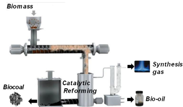
**Figure 1: Thermo-catalytic reforming (TCR) technology**
