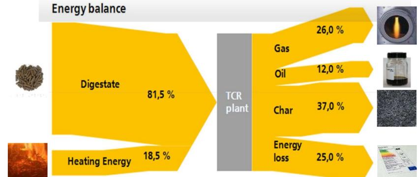
**Figure 2: The energy balance of the TCR process**
