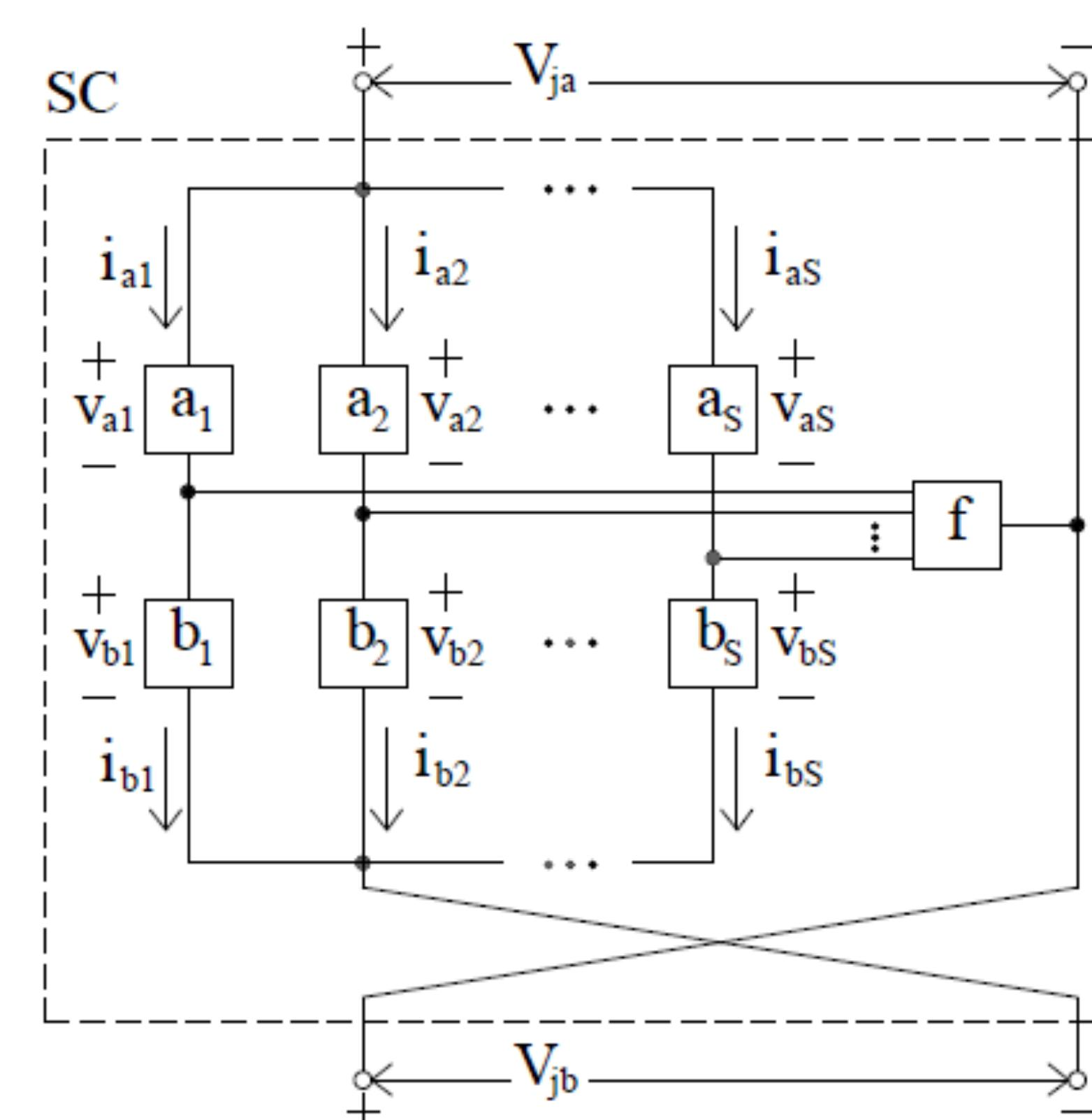
(b) Inverting buck-boost DCMMC
