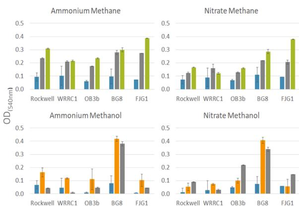
Biomass accumulation in different methanotrophic strains under different nitrogen/carbon conditions, with carbon provided at either 0.5 mmol, 1 mmol, 2 mmol, or 2.5 mmol per 100 ml of liquid cultures.
