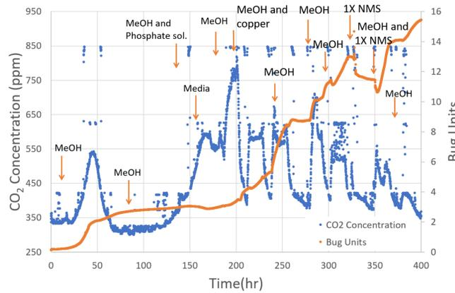
Effect of copper and nutrient addition on growth of *M. album* BG8 in a fed-batch process.
