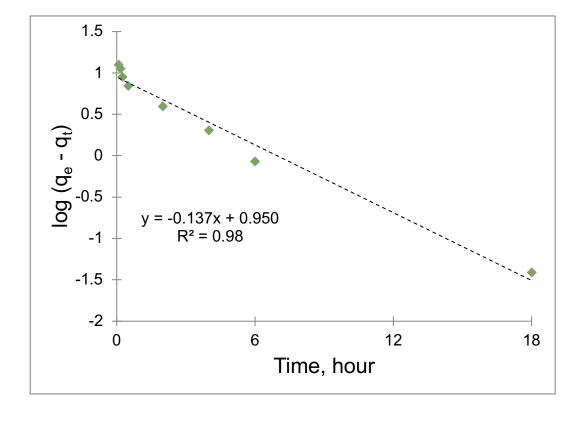
Fig. 5. Pseudosecond order kinetic model for adsorption of AEF onto CX5.5, 3 g/L dose.
